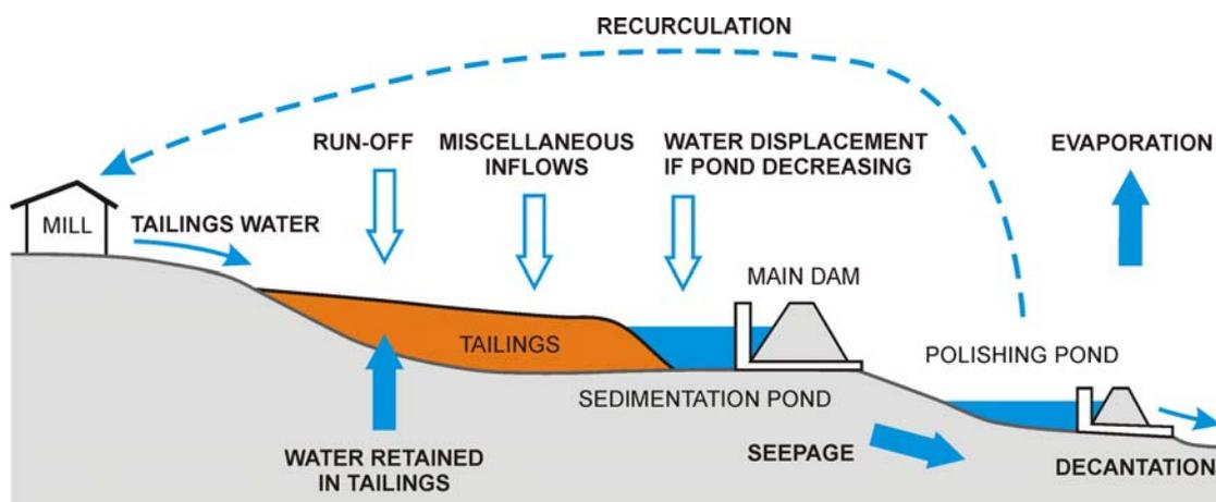
Figure 1: Hydrological cycle of a Tailings Disposal Facility.
